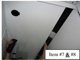
Slide the ceiling sections out of the way in order to access A/C hoses, wires, etc.
